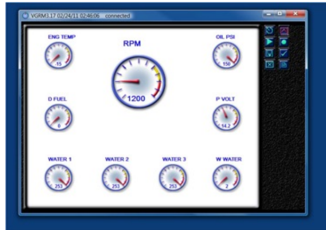
vDash receiving NMEA 2000 data directly from SeaSmart.Net adapter via Ethernet connection
